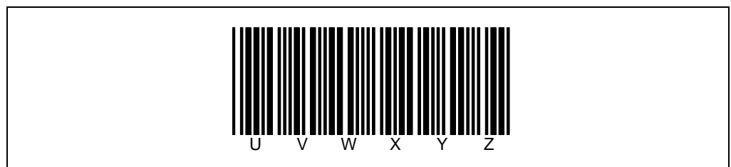
Fig. 6-1: Bar code pattern (code 39; module width 0.5 mm (19.7 mil); print ratio 2:1)
